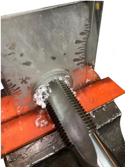
Hand threading cap holes
