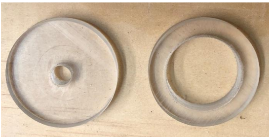
The rough cut disc (left) and machined part (right)
