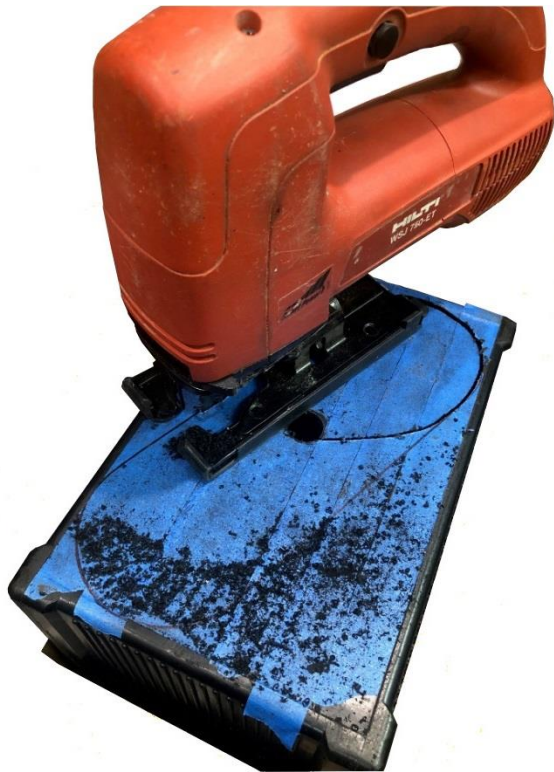
Cutting the opening in the original battery case bottom
