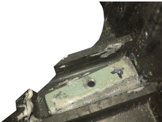
Capture nut epoxied inside the bottom of the battery case
