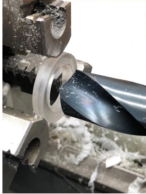
Drilling the \frac{59}{64} " pilot hole for the cell screw cap.
