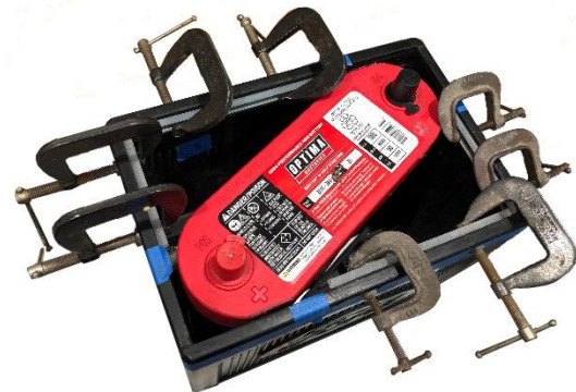
Edge supports for battery top cover
