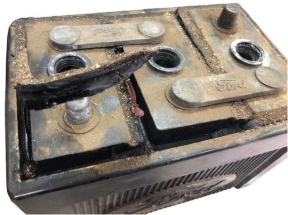
Tar being removed between cell covers
