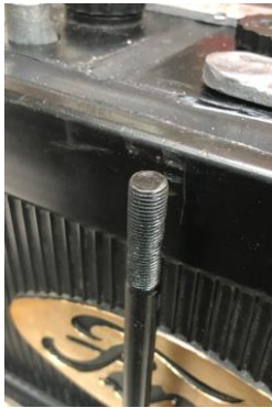
Hold down arm extensions and washers
