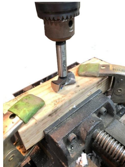
Drilling 1-3/8" hole in battery cover
