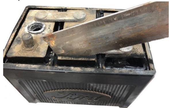
Cutting the cell tops for access
