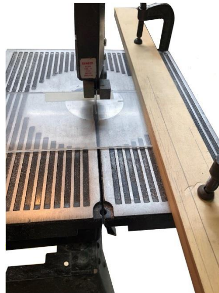
Cutting plastic parts
