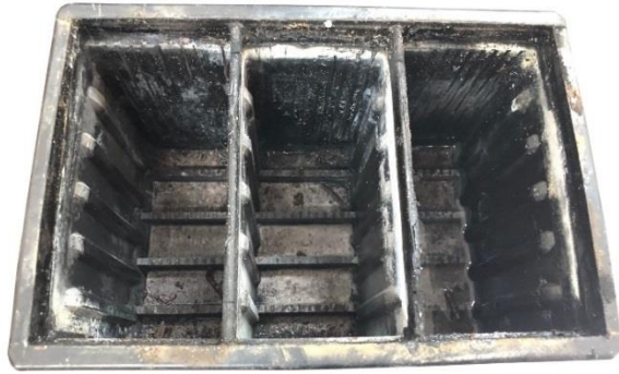
The empty battery case with cell dividers intact
